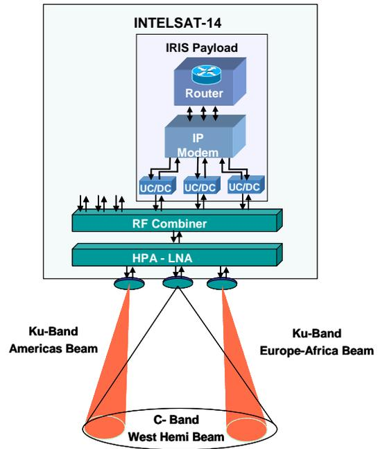
**Figure 2 - IRIS Payload Architecture**
