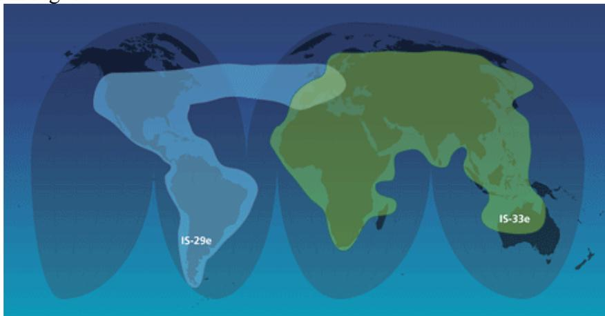
**Figure 1. Coverage for Intelsat-29e and Intelsat-33e<sup>§</sup>.**
