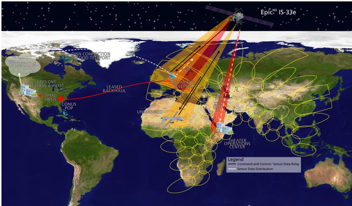
*Fig 5: Example future IGC Unmanned ISR Network*
