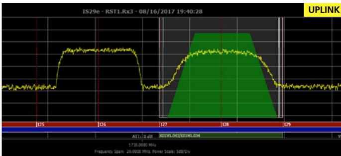
Fig. 11: IS-29e Reconfigured to Terminate Interferer & Reallocate Friendly Carrier
