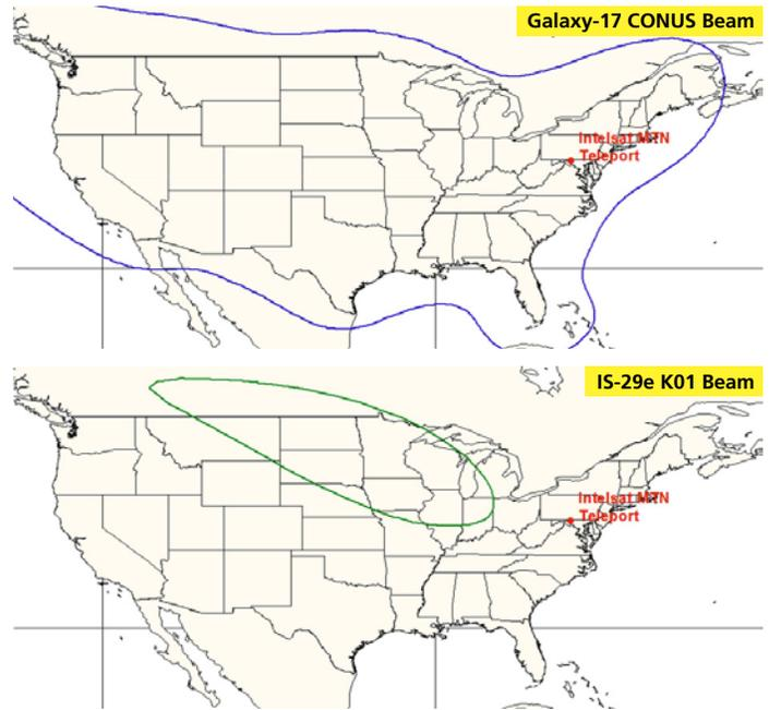
Fig. 1: Wide Beam versus Spot Beam Coverage Areas
