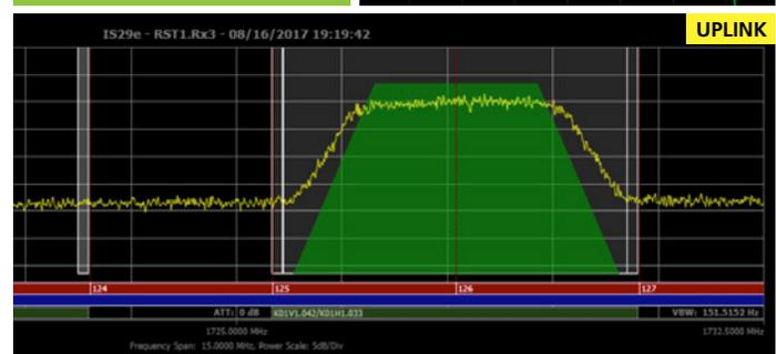
Fig. 8: Simultaneous Friendly and In-Beam Interferer Transmissions
