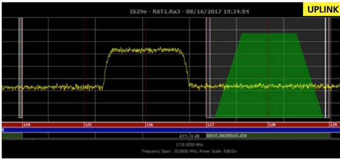
Fig. 9: IS-29e Reconfiguration to Terminate Interferer & Reallocate Friendly Carrier
