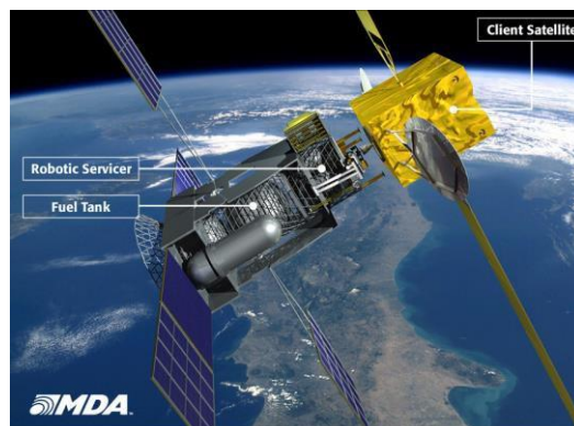
Figure 2: Satellite In-orbit Servicer (SIS) docked to Client Satellite [MDA]
