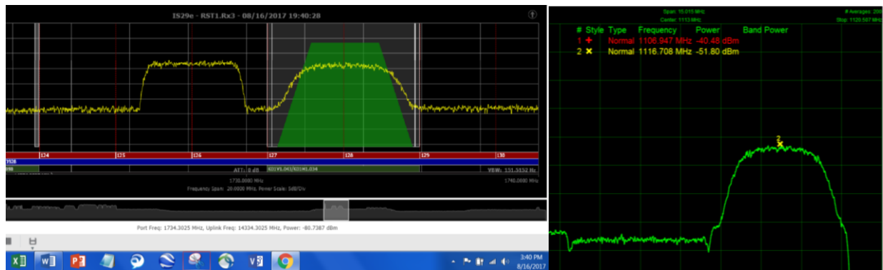
Figure 12 –IS-29e Reconfiguration to Terminate Interferer & Reallocate Friendly Carrier
