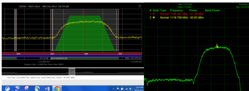
Figure 7 – Nominal Uplink & Downlink Spectrums for In-Beam Interferer Testing
